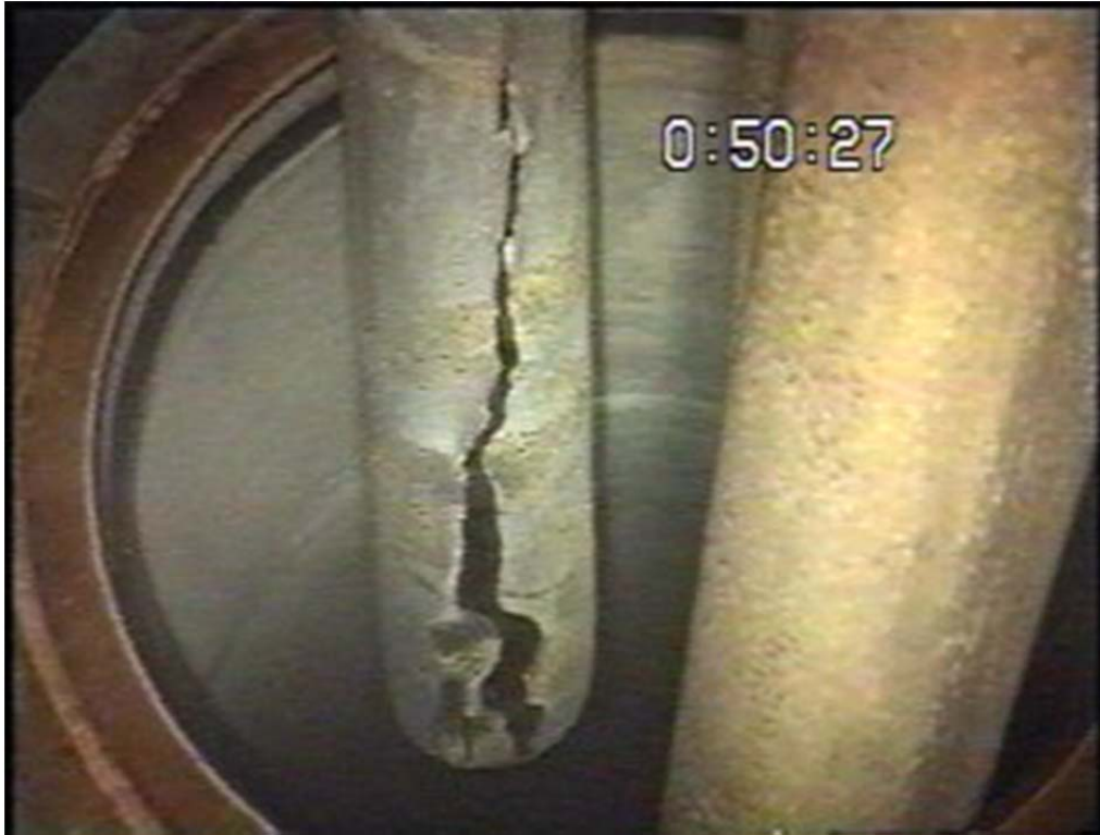
Figure 8. Cracked Z can inside an HWCTR oversized can.
