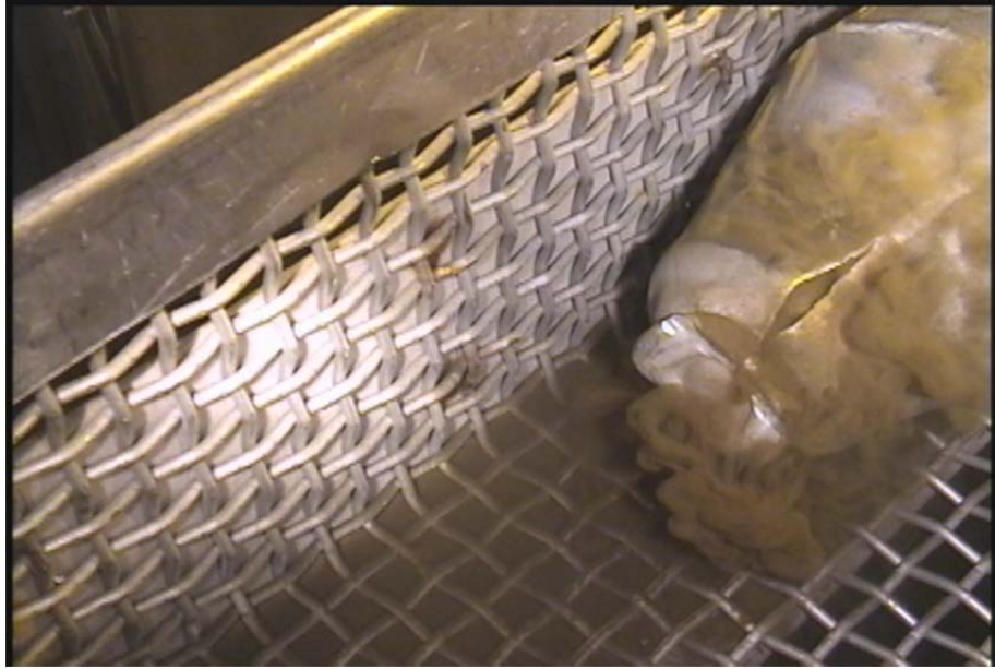
Figure 9. Sealed tube with crack at bottom.
