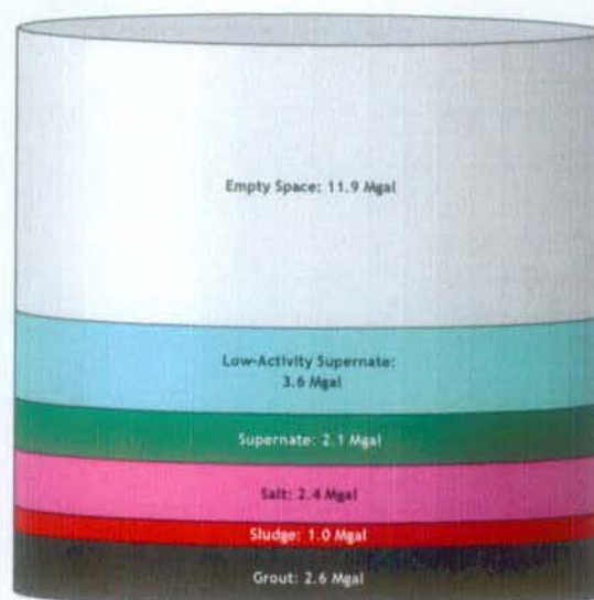
Figure 2: Current Old-Style Tank Contents
