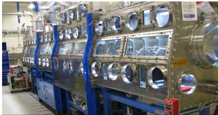
Glovebox Line 1 of the Recovery Glovebox Line (Source: 33 rd Annual Report to Congress)
