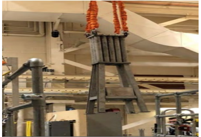
Annular Core Research Reactor fuel element rack lifted over the reactor pool. (Source: 33 rd Annual Report to Congress)
