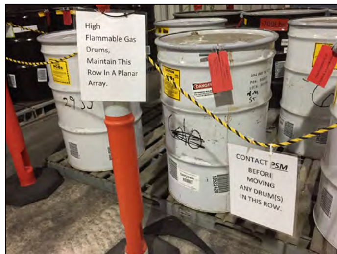
Figure 2. Staging area for waste drums known to have elevated levels of flammable gas
