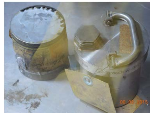
Examples of storage containers and conditions for nuclear materials in the Plutonium Facility
