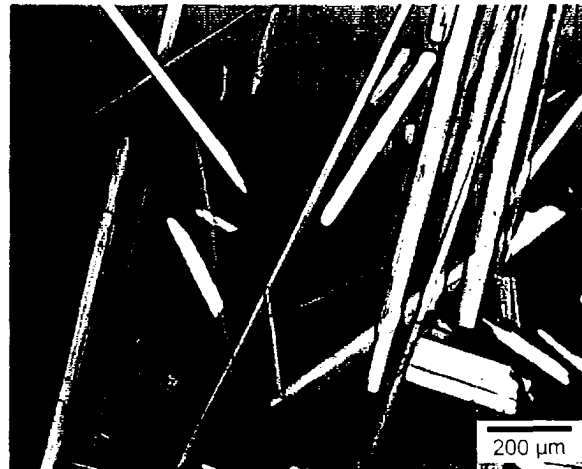
Figure 3-3. Sodium Phosphate Crystals from Tank S-102 (Colors Due to Use of Polarized Light with Red I Compensator).
