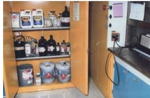
Flammable storage cabinet at INEEL
