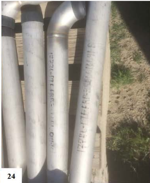
Figures A-23 to A-25. Staff review team photographs illustrating illegible physical markings of SSCs at the MHF Laydown Yard.
