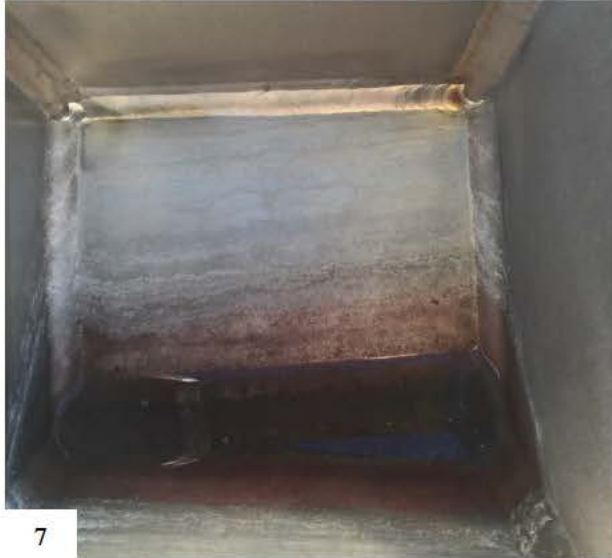
Figures A-7 to A-8. Staff review team photographs illustrating deficient storage conditions at the MHF Laydown Yard. Figure A-7 shows water accumulated inside a vessel. Figure A-8 shows additional pipe modules buried in the sand.
